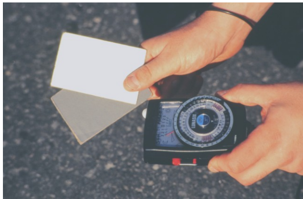
Figure 4.1 - Cut pieces of Kodak's Gray Card, colored grey on one side and white on the reverse, for measuring various surfaces in different areas using a good light-meter.
