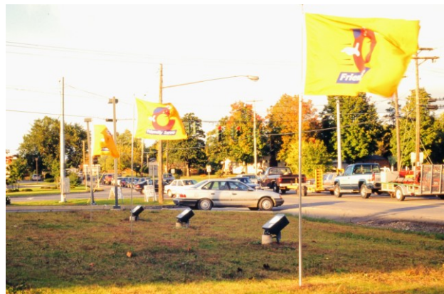
Figure 4.35 - A lighting contractor had free reign to illuminate a company's flags in this small town in upstate New York in the mid 1990s. The ground-mounted HPS lamps were an incredible 400 watts and each one polluted like twenty 400 watt FCO street-light counterparts (5% for urban summer).
