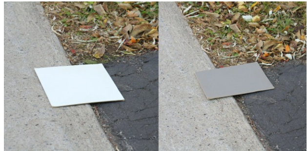
Figure 4.3 - The two sides of Kodak's Gray Card. The white, slightly aged side has a reflectivity of about 85%, and the grey side is 18% reflective. Part of an over-coated black asphalt driveway is on the right, while a concrete sidewalk is at left.
