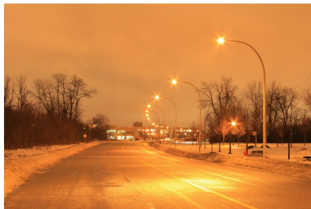
Figure 5.21 - Fresh and intense HPS cobra-head lighting of the past, associated with glare, light spill and a bright overcast.
