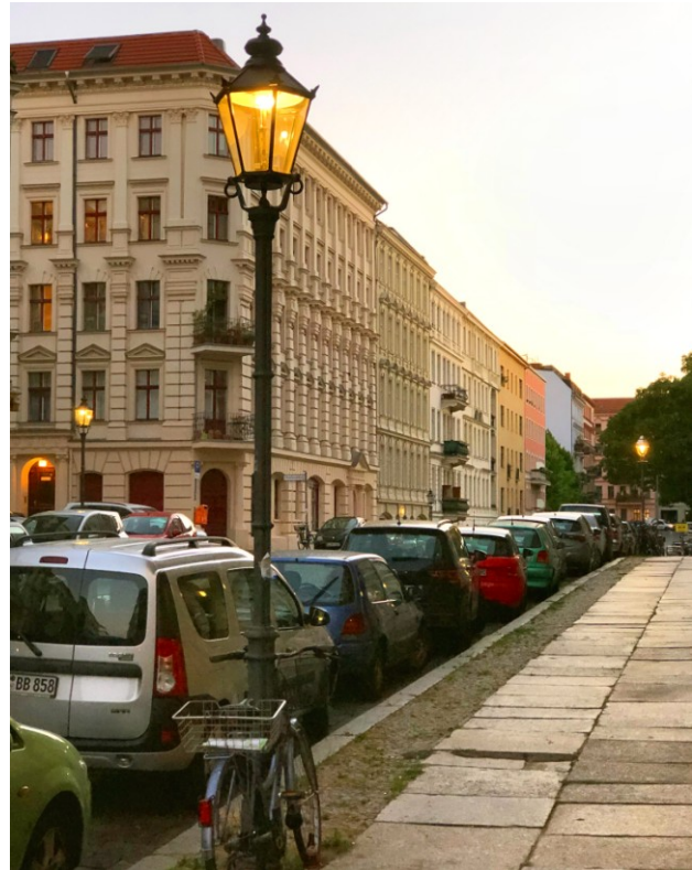
Figure 2.5 - Dating back to 1892-93, these are some of the original double-mantled "Model Lamp" style gas-lanterns operating in Kreuzberg, Berlin. Converted now to run with 4 mantles, this image was obtained in 2018. Photo by C. Fraser.
