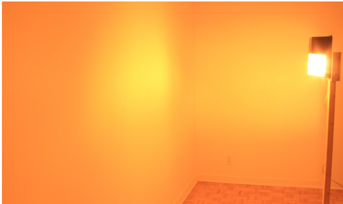
Figure 3.67 - A typical mini HPS wall-pack or side-pack made by numerous companies, these utilize medium socket lamps of between 35 and 150 watts. This one contains a ballast for a 70 watt lamp and a well used HPS lamp is installed. A rather poor lighting pattern is shown for the light distribution, much of it being shed straight out horizontally.
