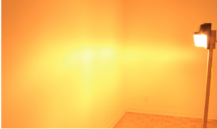
Figure 3.66 - Here is an older HPS wall-pack made sometime in the 1980s by Holophane. A used 70 watt mogul sodium lamp is installed. The wall-pack employs a thick glass refractor cover and the lighting pattern shows that a significant portion of the light is thrown at an angle of 65° to 80° above the nadir.
