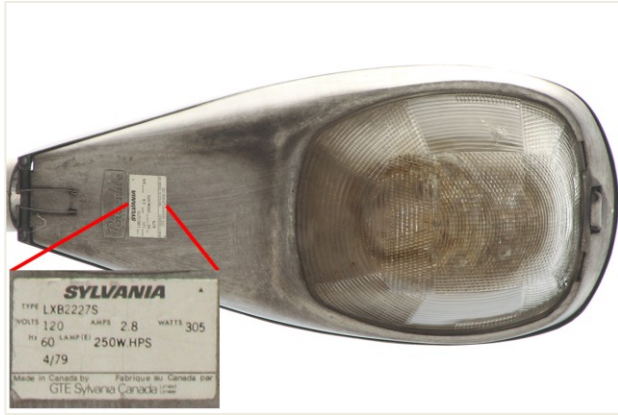
Figure 5.20 - With a manufacture date of April 1979, this 250 watt HPS cobra-head served an industrial road for 38 years. Incredibly, when retired in 2018 it was replaced with a warm-toned GE Evolve LED FCO head with just 31 system watts.
